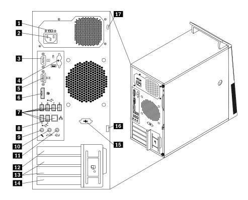
Figure 2. Rear connector locations
